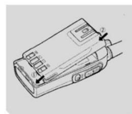
Match the back of the battery pack with the corresponding guides on the back of the transceiver.
