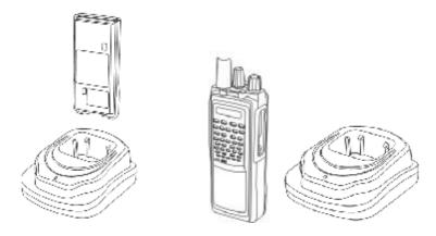
The first charging after purchase or after long time storage (longer than two months) may make the battery pack unable to reach its normal capacity. After repeated charging for twice or more, its capacity will recover to the normal value.
