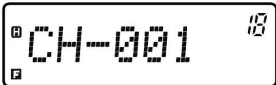
9. Shortly press the [Function button] to confirm and save the desired values and enter the channel name entry status.
