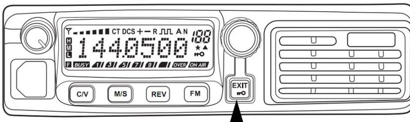
2. Once again press [EXIT] for 2 seconds to release the key locking.
