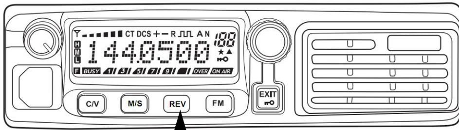
When the reverse frequency function is activated, the symbol “R” will appear on the display screen.
