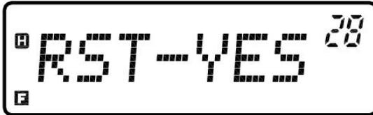
5. Shortly press the [Function button] to confirm and save the desired values. Or shortly press [
