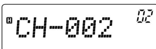
2. Rotate the [Tuning knob] to select the desired memory channel number.
