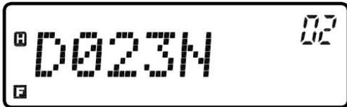
5. Shortly press the [Function button] to confirm and save the desired values. Or shortly press [
