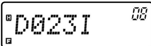
5. Shortly press the [Function button] to confirm and save the desired values. Or shortly press [
