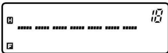
10. Shortly press [C/V] to select character. Rotate the [Tuning knob] or press [UP]/[DWN] on the handheld MIC to select the desired symbol
